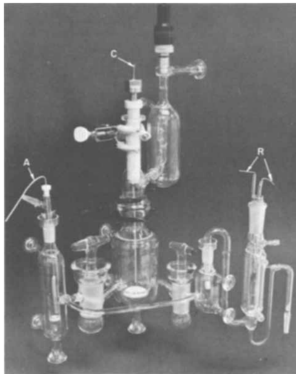
Fig. 1. Electrolysis cell; A, anode; C, cathode; R, reference electrodes.
