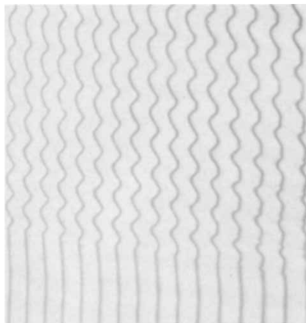
Fig. 4. Multiple beam interferogram of an etched InSb single crystal. The periodic deflections of the interference fringes in the upper part reflect the impurity concentration fluctuations always present under seed rotation. The homogeneous impurity distribution in the lower part (straight line interference fringes) reflects the growth conditions associated with crucible rotation without seed rotation. Magnification 230X.
