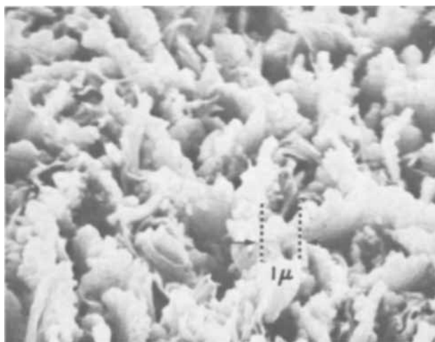
Fig. 8. Copper surface after peeling from treated polysulfone
