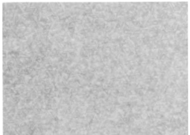
Fig. 6B. Layer 3 \mu thick, cooled from growth temperature at 0.8°C/min, showing absence of cracks. Magnification 100X.
