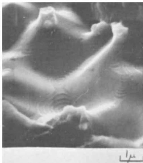
Fig. 1. Metal surface, observed at a tilt of 30°, showing terracing, beneath an oxide layer where this has spalled away from a specimen of an Fe-19% Cr alloy during cooling after oxidation at 950°C for 6 hr in pure oxygen.
