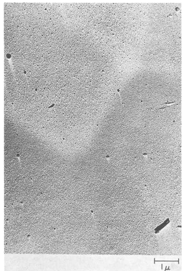
Fig. 8. Electron micrograph of a vitreous boron filament
