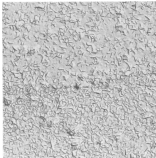
Fig. 2. Top surface of a film formed on magnesium in 100 min in pure water. Magnification 15,000X.
