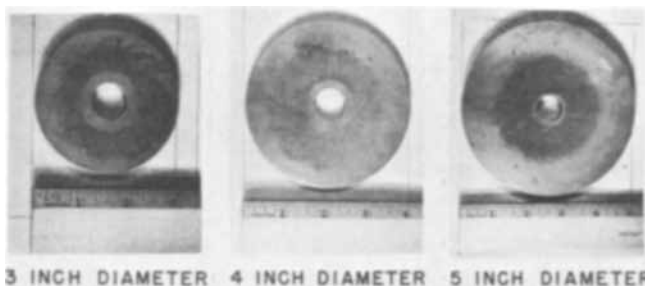
Fig. 4. Distribution of corrosion on cast iron disks of different diameter rotated in sea water at the same speed in revolutions per min: cast iron disks rotating spindle test 30 days at 15°C.
