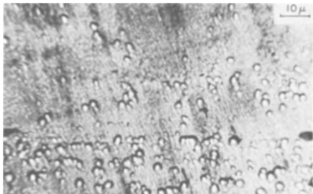
Fig. 9. Etch figures on a surface parallel to the growth direction for an In:InSb growth experiment.
