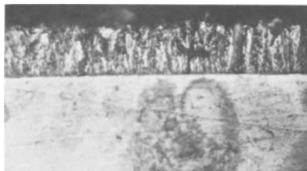
Fig. 2. Cross section of titanium diboride coating on molybdenum. Deposit is 2.3 mils thick and has columnar structure. Magnification approx. 430X.
