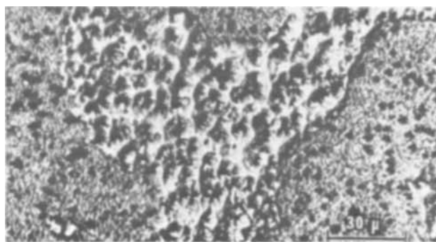
Fig. 9. Etched surface texture after dissolution of 99999 copper in the active mode (2M \text{KNO}_3 , 50 \text{A}/\text{cm}^2 , 2500 \text{cm}/\text{sec} ).
