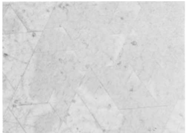
Fig. 6A. Cracks in ZnSe layers grown on Ge: layer 30 \mu thick, cooled from growth temperature at 10°C/min, showing crack formation. Magnification 300X.
