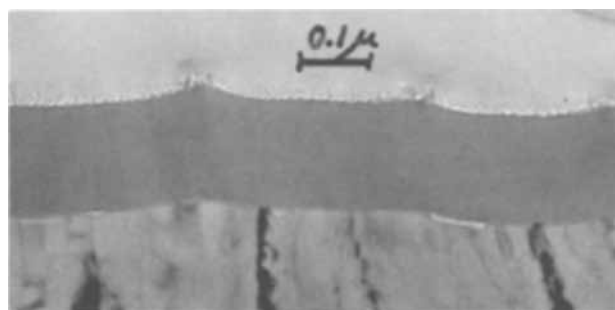
Fig. 4. Cross section of 50v barrier layer coating at 84,000 magnification.
