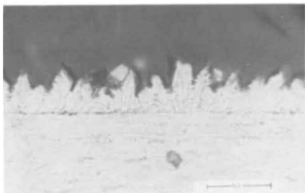
Fig. 4. Photomicrograph of zinc deposit produced by pulsed current charging. Current density 80 \text{ ma/cm}^2 , time on 10 msec, time off 10 msec, quantity of charge passed 60 \text{ coulombs/cm}^2 , current efficiency for deposition 85%.
