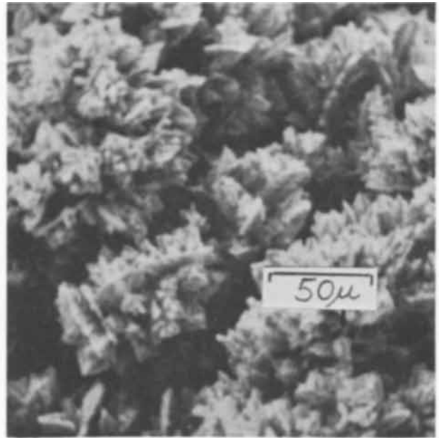
Fig. 11. Scanning electron micrograph of morphology at Re = 13,500 , 1 min at 1600 \text{ amp/m}^2 viewed at 45^\circ (X400).
