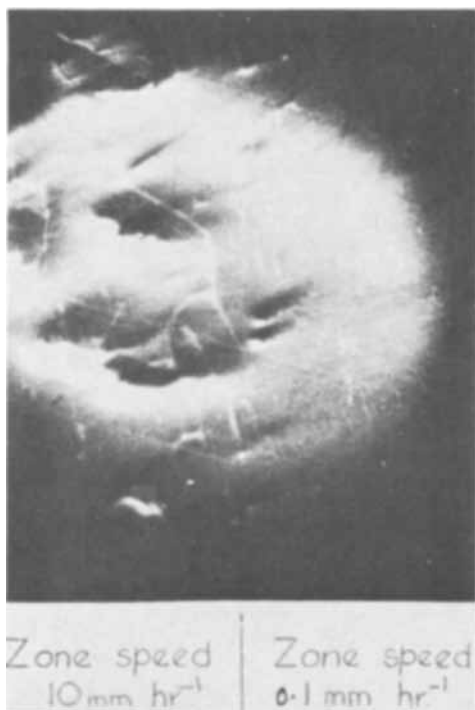
Fig. 3. Photomicrograph of the surface of a zone refined ingot of nominal composition \text{ZnCdSn}_2\text{As}_4 showing that the second phase present when the zone speed was 10 mm/hr and disappeared when the speed was reduced to 0.1 mm/hr. Magnification approx. 150X.
