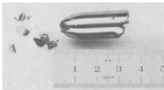
Fig. 3. Boule of vapor grown ZnTe crystal
