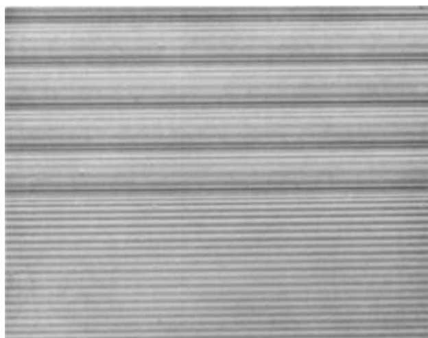
Fig. 3. Growth characteristics of the off facet region of InSb as revealed by vibrational "rate striations." The upper part, grown with seed rotation and synchronized crucible rotation exhibits periodic growth rate changes as seen from the varying spacing of the "rate striations." The lower part, pulled with crucible rotation only, exhibits a constant growth rate (constant spacing of "rate striations") which is a prerequisite for homogeneous impurity incorporation. Magnification approx. 450X.
