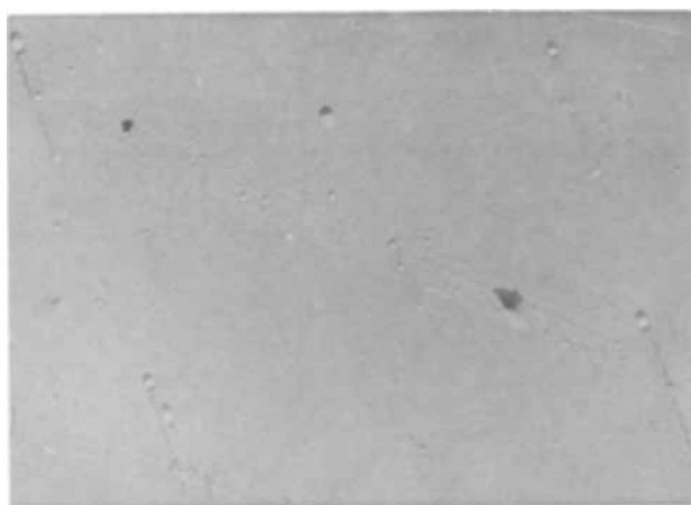
Fig. 7. Slip lines in germanium wafer \langle 110 \rangle , direction \langle 110 \rangle as seen at the electron microscope. Magnification 9750X.
