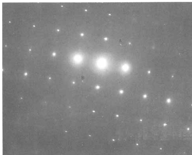
Fig. 1. {100} diffraction pattern of as-grown PbSe. Extra spots at points A and B may be due to precipitated Pb.
