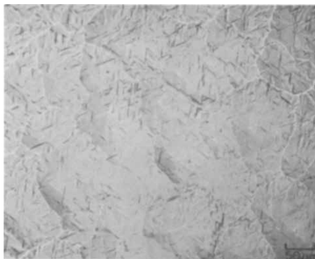
Fig. 3. The surface structure of a 30- \mu m GaAs film growth on (0001) Al 2 O 3 .
