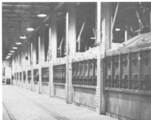
Fig. 2. A group of high-tension separators which make an electrodynamic concentration of iron ore at the rate of 1000 tons/hr.
