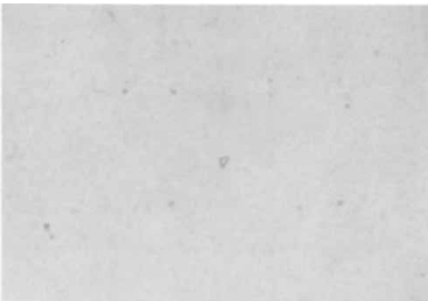
Fig. 3B. Ge surface after removal of ZnSe layer in Fig. 3A, showing that the original mirror polish is retained. Magnification 300X.
