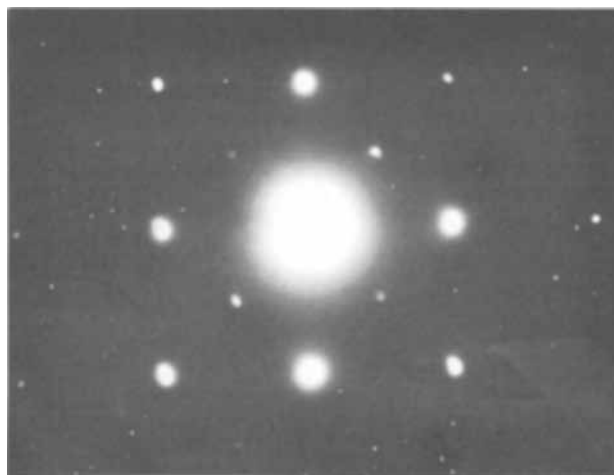
Fig. 1. Transmission electron diffraction pattern of GaAs films grown on semi-insulating GaAs substrate of (100) orientation.
