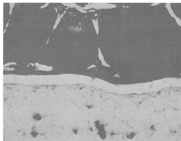
Fig. 5. Photomicrograph of niobium sample coated with 14 \mu of molybdenum.
