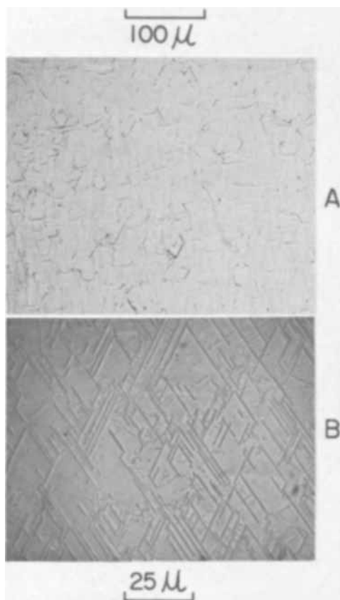
Fig. 3. Defect structure in a Ge film on a (0001) oriented sapphire substrate: (a) as-deposited (175X), and (b) etched surface. Magnification approx. 400X.
