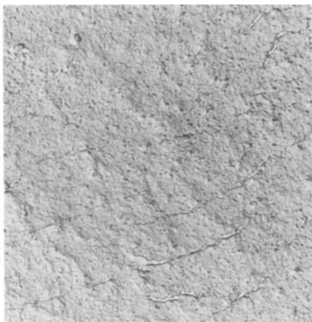
Fig. 3. Top surface of a film formed in 68 hr in a 10^{-3}\text{M} \text{NaIO}_4 solution, pH 10. Magnification 15,000X.
