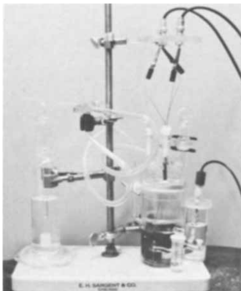
Fig. 1. Double layer capacitance measurement cell configuration
