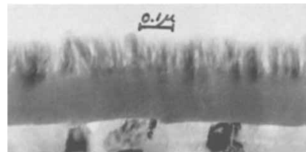
Fig. 5. (a, top, and b, bottom). Cross sections of 100v barrier layer coatings at 84,000 magnification.
